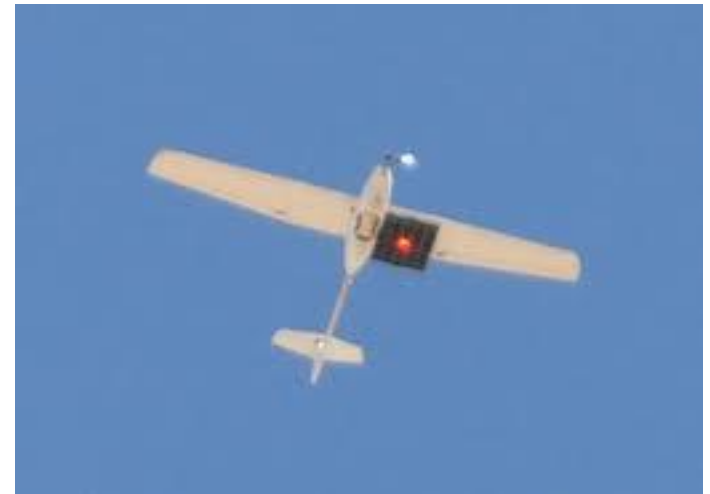
LaserMotive outdoor laser power to UAV (2012)
