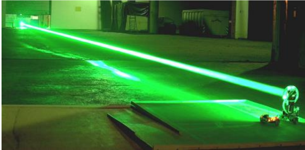
EADS Astrium tracking laser to power rover (2003)
