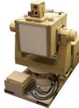
Solid State Based 7 kW Transmitter at 92 GHz
