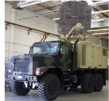
TWT Based 100 kW Transmitter at 92 GHz
